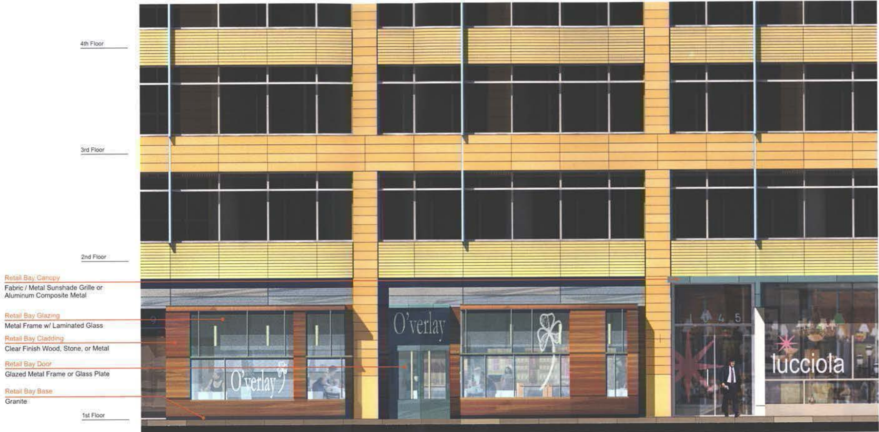
Enlargement View - East Elevation of West 4th Street Office Building Refer to Sheet 4.2
